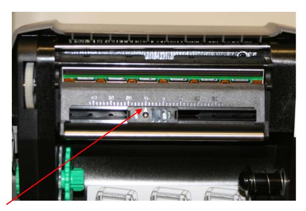
**VERY IMPORTANT!** Your printer has two sensors that make sure your tags always print in the right place, and they must be precisely aligned to work correctly. The Upper and Lower Sensors (indicated by the red arrows) were adjusted and calibrated for your tags and/or labels before your printer was sent to you. **DO NOT MOVE OR ADJUST** the sensors in any way unless specifically instructed to do so *by an Arch Crown Technician*.
