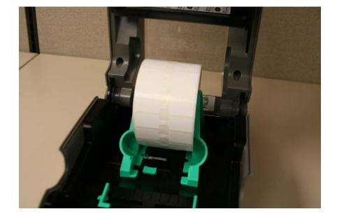
10. Pull the free end of the labels towards the front of the printer, through the adjustable guides near the front of the printer, then over the rubber roller, and out the front. Make sure that the guides are adjusted to hold the labels straight. Close the cover of the printer, making sure that it locks in the down postion.
