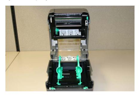
2. The thermal transfer ribbon (ink) will be loaded into the printhead mechanism contained in the cover, as shown in the photo below:
