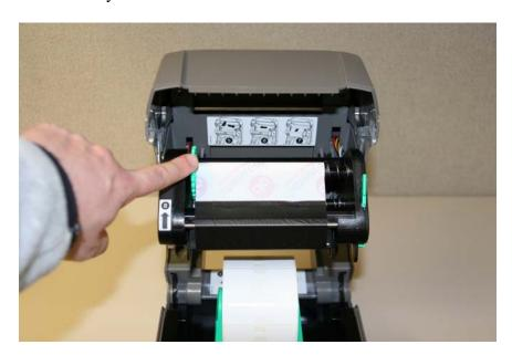
9. You can now load your new roll of labels between the green brackets in the base of the printer. The brackets are spring-loaded, and will automatically adjust to firmly hold your label roll.
