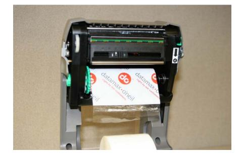
4. Release the printhead mechanism by pushing down in the direction of the arrow.
