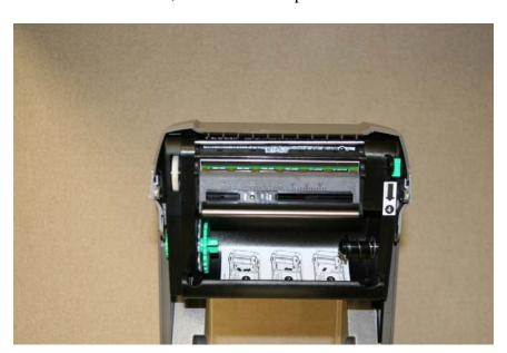
3. Insert the new ribbon onto the spindles as shown; black spring-loaded spindle on the right, and green wheel on the left. Push the ribbon completely over the notches on green left-hand wheel. NOTE the direction of the ribbon – the loose end of the ribbon should come off the front of the roll, with any printing (e.g. "datamax-o'neil") on the roll facing you.
