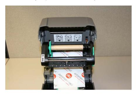
7. Now, take the loose end of the new ribbon, wrap it around the front the of printhead mechanism and fasten it to the empty cardboard core with a piece of tape.
