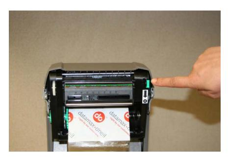
5. There will be an empty cardboard ribbon core included with your new ribbon. With the printhead in the open position, note the two spindles in the upper part of the mechanism. Insert the new core onto the spindles; first onto the springloaded spindle on the right...
