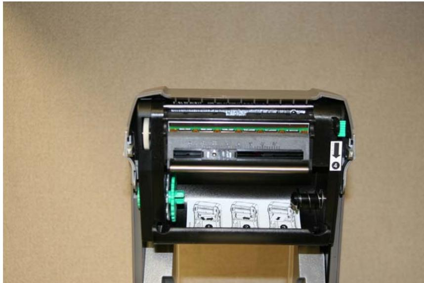
3. Insert the new ribbon onto the spindles as shown; black spring-loaded spindle on the right, and green wheel on the left. Push the ribbon completely over the notches on green left-hand wheel. NOTE the direction of the ribbon – the loose end of the ribbon should come off the front of the roll, with any printing (e.g. “datamax-o’neil”) on the roll facing you.
