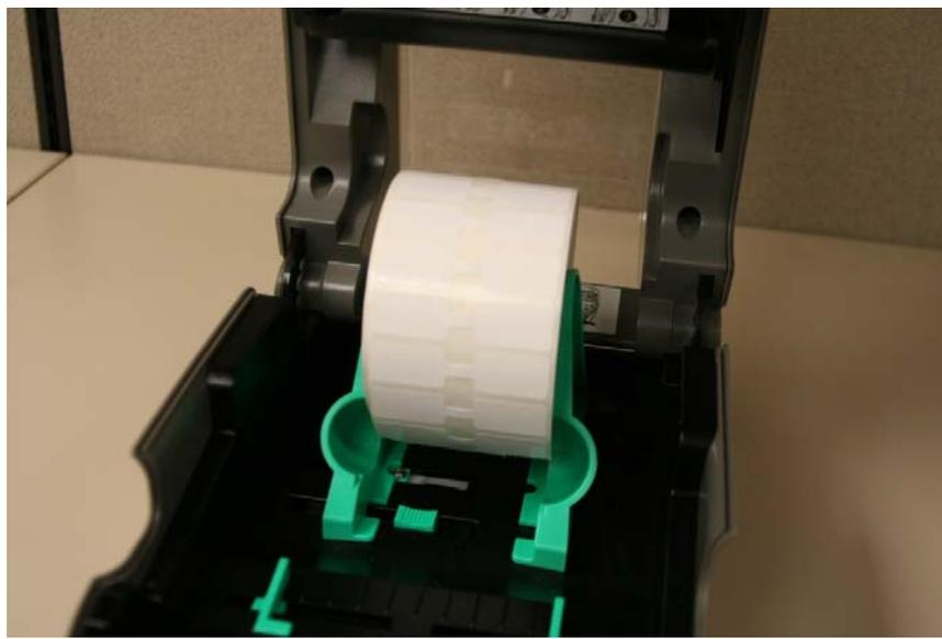
10. Pull the free end of the labels towards the front of the printer, through the adjustable guides near the front of the printer, then over the rubber roller, and out the front. Make sure that the guides are adjusted to hold the labels straight. Close the cover of the printer, making sure that it locks in the down position.
