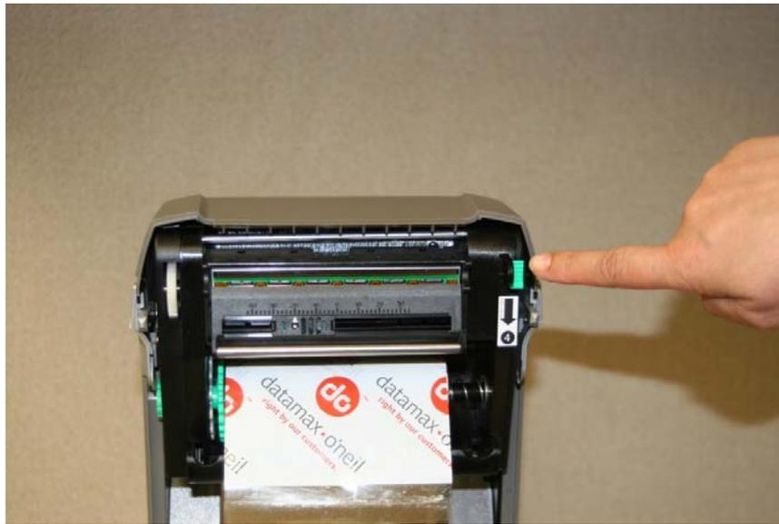
5. There will be an empty cardboard ribbon core included with your new ribbon. With the printhead in the open position, note the two spindles in the upper part of the mechanism. Insert the new core onto the spindles; first onto the spring-loaded spindle on the right...
