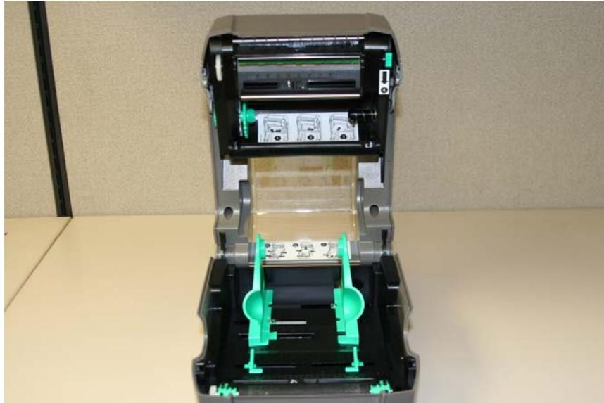
2. The thermal transfer ribbon (ink) will be loaded into the printhead mechanism contained in the cover, as shown in the photo below:
