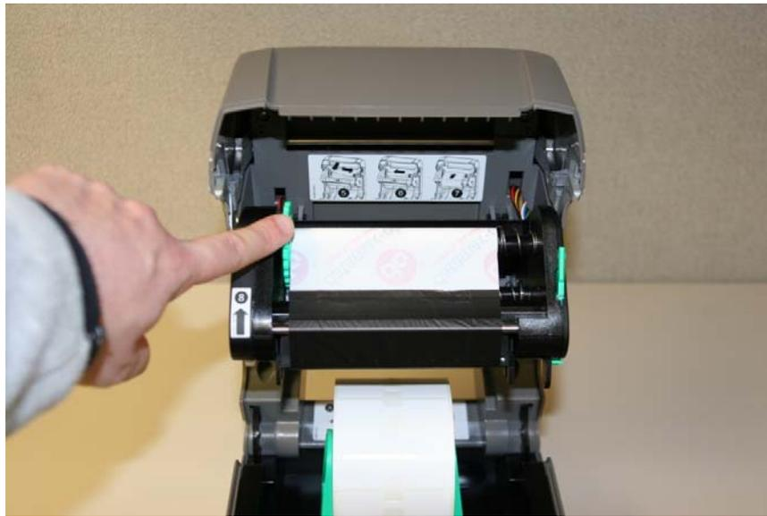
9. You can now load your new roll of labels between the green brackets in the base of the printer. The brackets are spring-loaded, and will automatically adjust to firmly hold your label roll.
