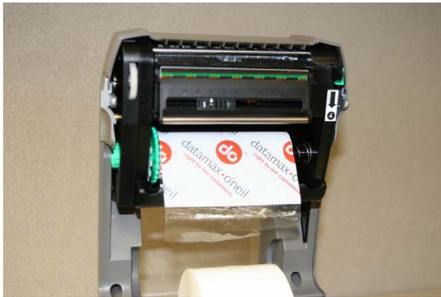
4. Release the printhead mechanism by pushing down in the direction of the arrow.
