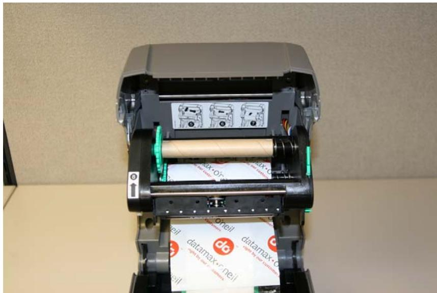
7. Now, take the loose end of the new ribbon, wrap it around the front the of printhead mechanism and fasten it to the empty cardboard core with a piece of tape.
